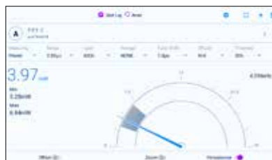
Analog needle display of power Persistence and min/max tracking.
