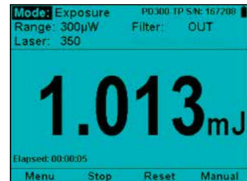
Exposure measurement (energy summing) with photodiode sensor.
