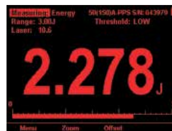
Bargraph display of energy. Colors set for work with protective glasses.
